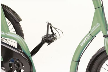
840 Pedal cages with straps. To keep the forefoot positioned on the pedal.
