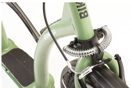
882 Steering limiter with spring.
